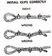
Correct way to apply U-bolts to form an eye in wire rope.
