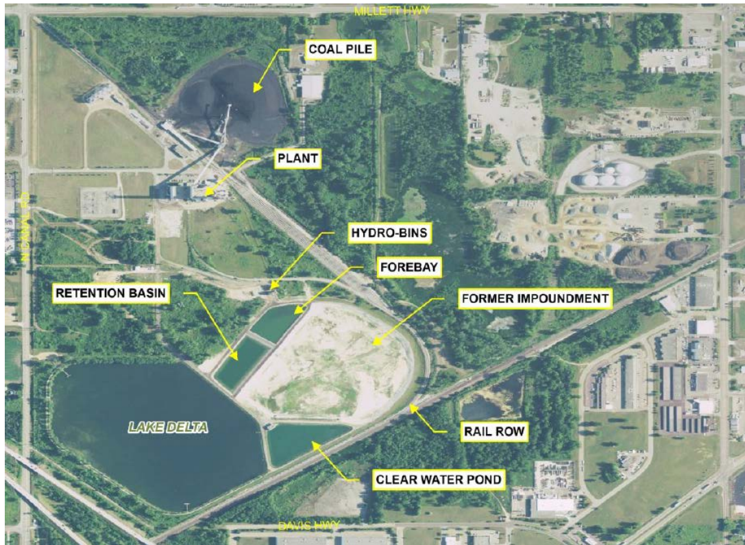
Figure 2. Erickson Power Station Site Configuration
