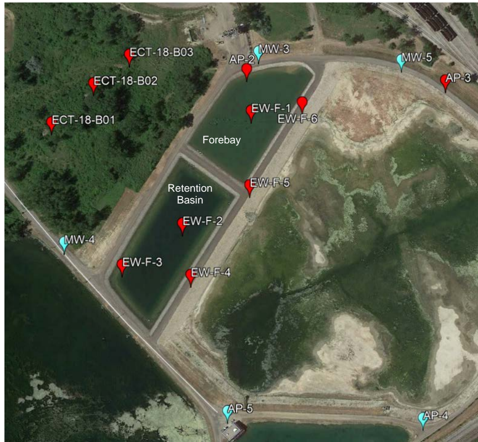
Figure 5. Approximate Boring/Monitoring Well Locations
