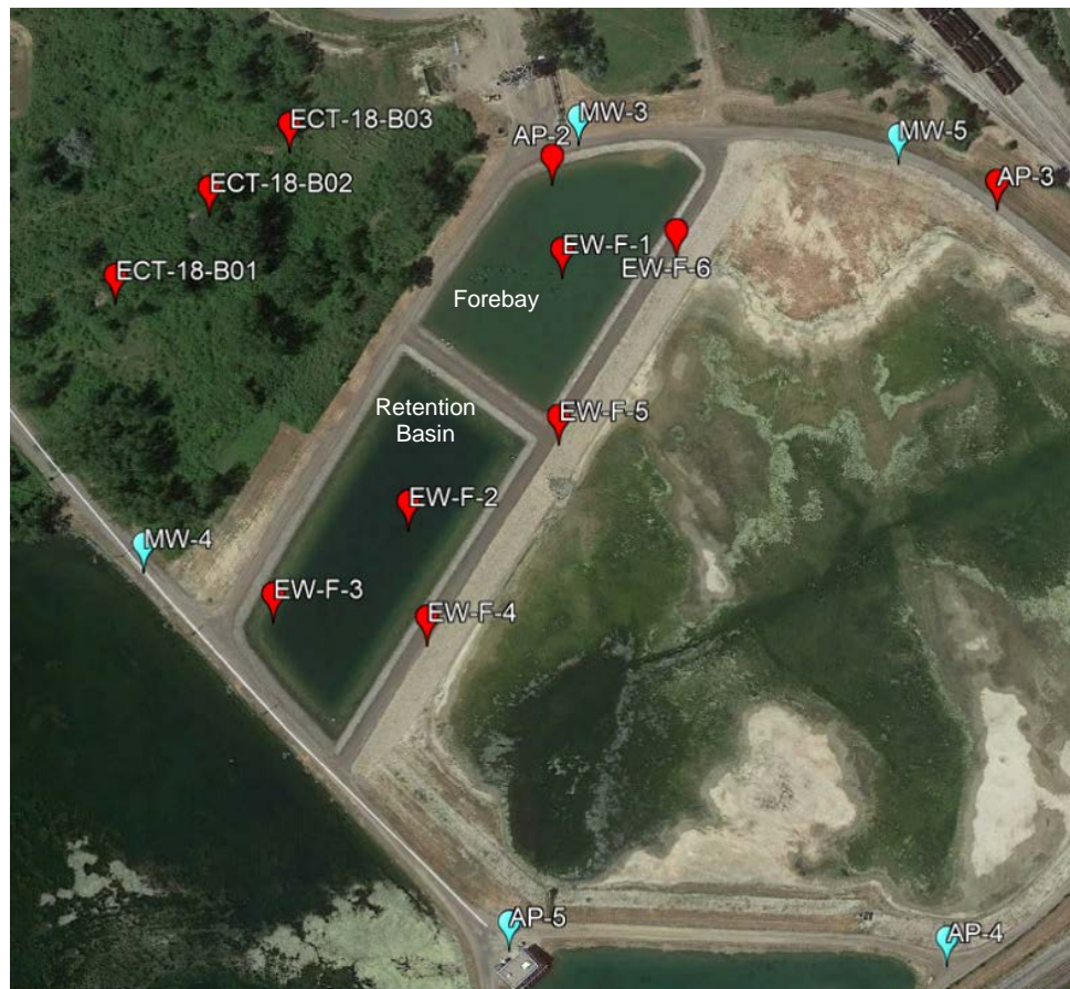
Figure 8. Approximate Boring/Monitoring Well Locations
