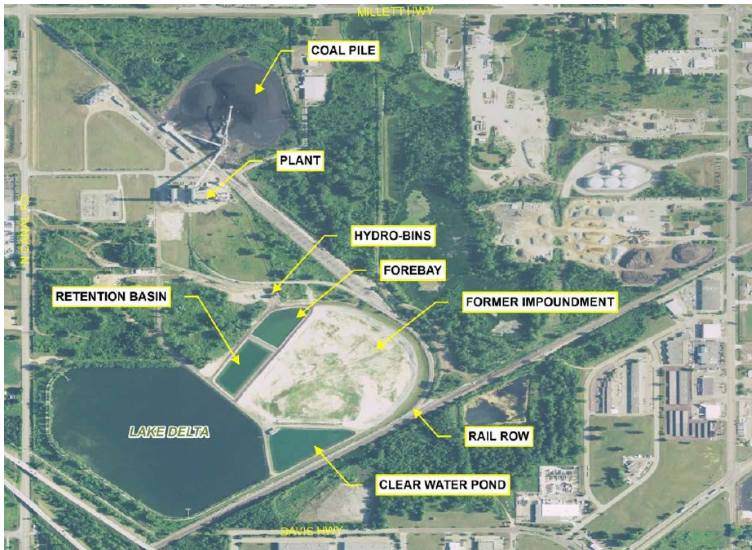
Figure 2. Erickson Power Station Site Configuration
