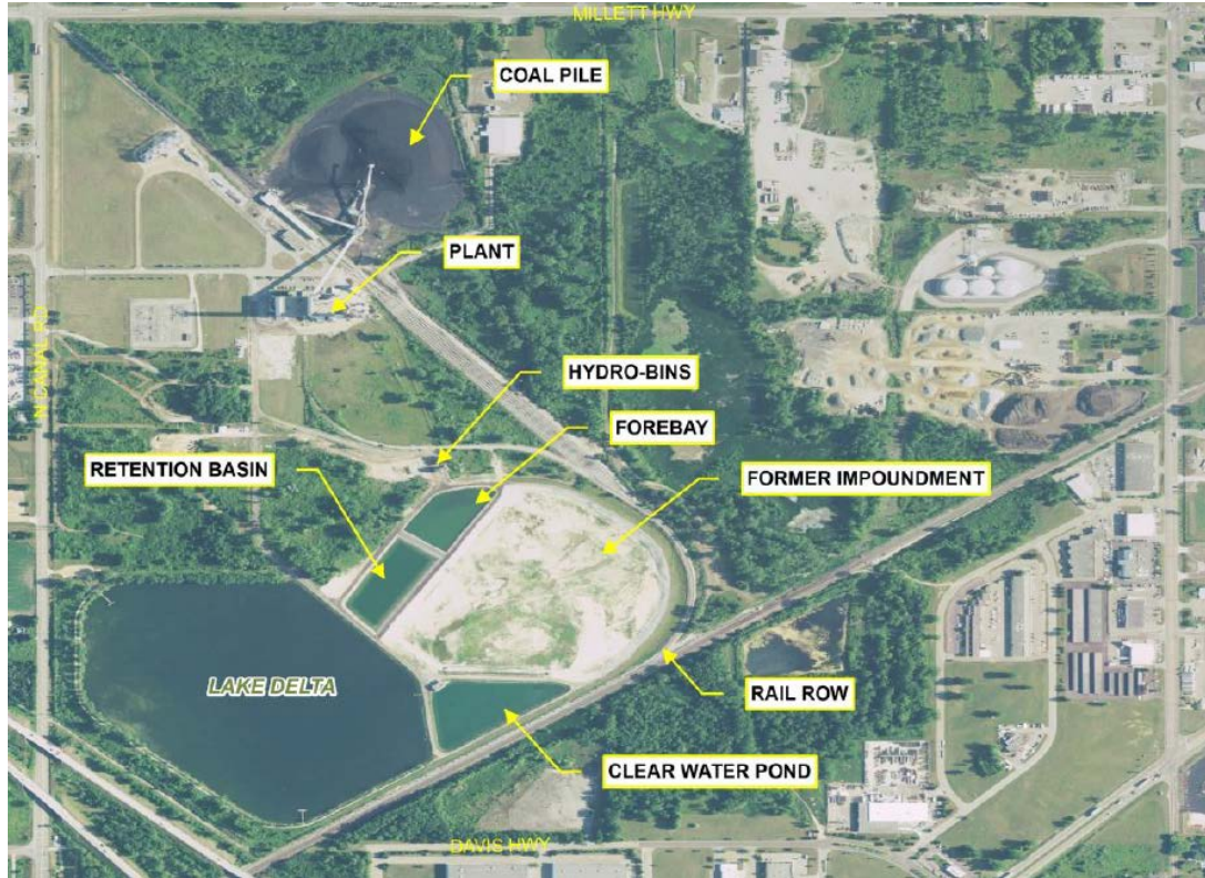
Figure 2. Erickson Power Station Site Configuration
