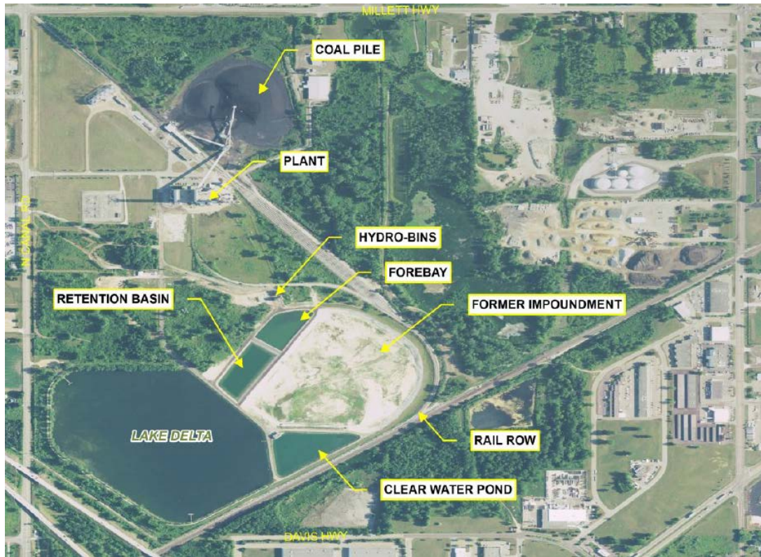
Figure 2. Erickson Power Station Site Configuration
