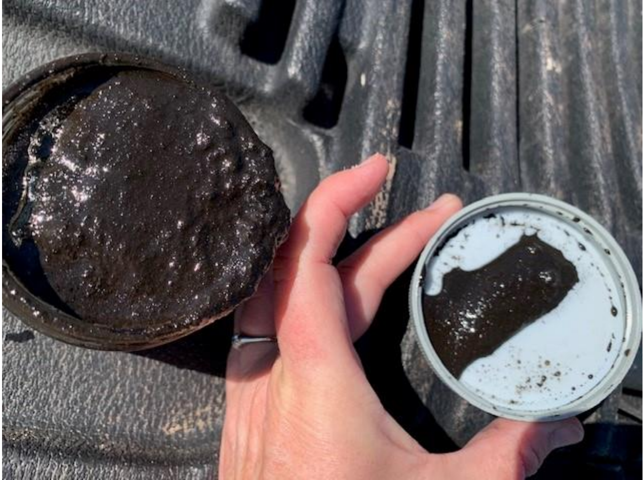
Figure 3. Ash collected from the floor of the Forebay
