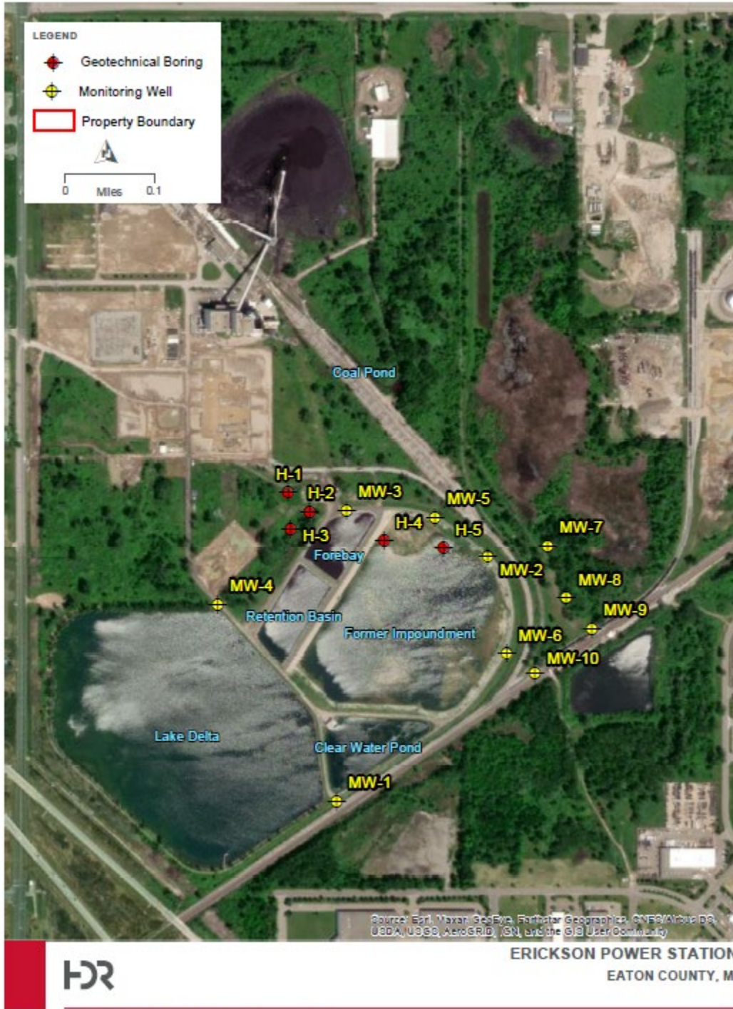
Figure 3-1. Geotechnical and Monitoring Well Borings Containing Lithologic Data for Use in Developing the Geologic Framework for the Groundwater Model
