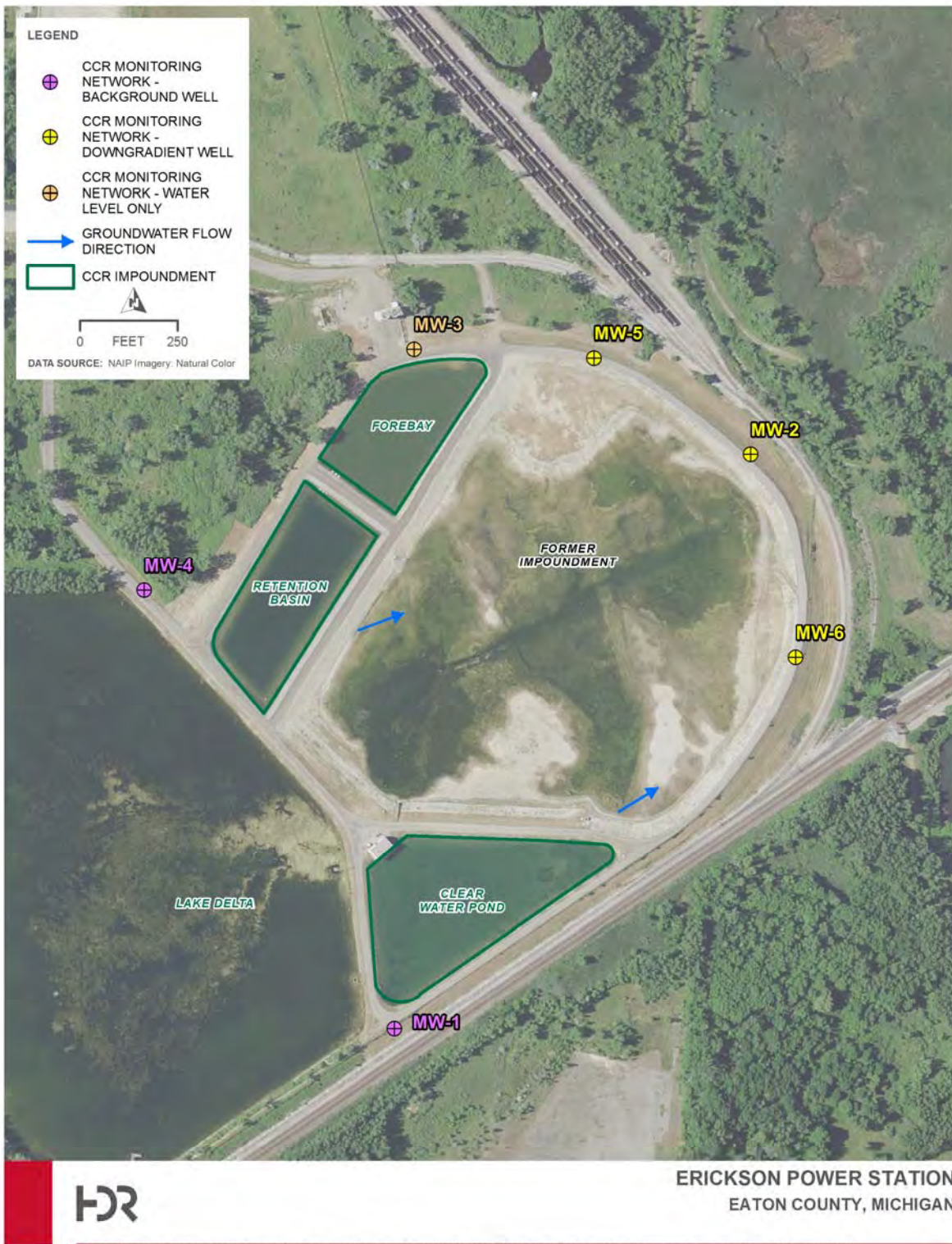
Figure 2. Erickson Power Station – CCR Unit and Monitoring Well Location Map
