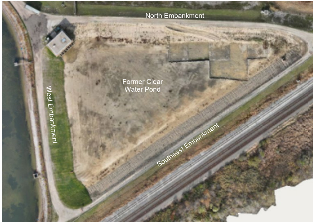
Figure 5. Former Clear Water Pond Embankment Terminology
