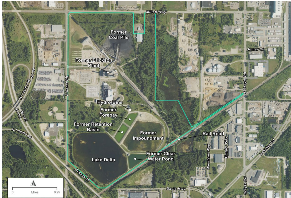
Figure 2. Former Erickson Power Station Facility Layout
