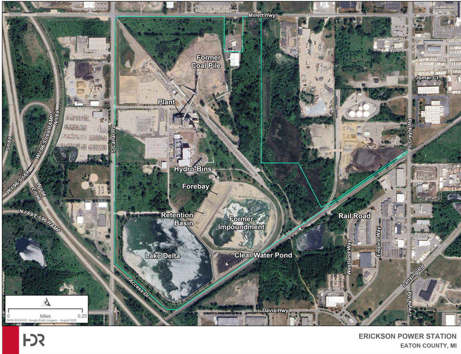
Figure 2. Erickson Power Station Facility Layout
