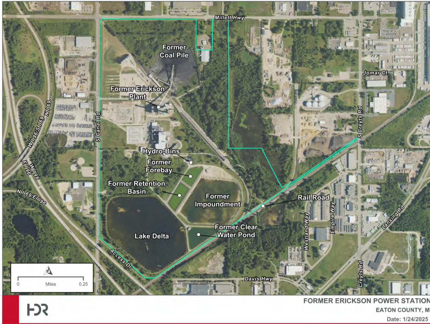
Figure 2. Former Erickson Power Station Facility Layout
