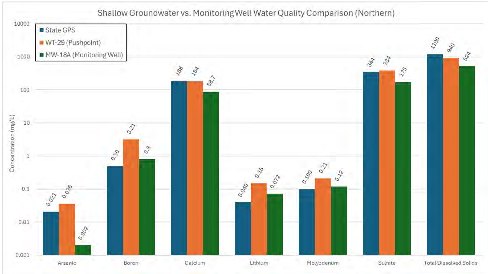
Figure 7. Pushpoint Sampler Groundwater vs. Monitoring Well Water Quality (Northern)
