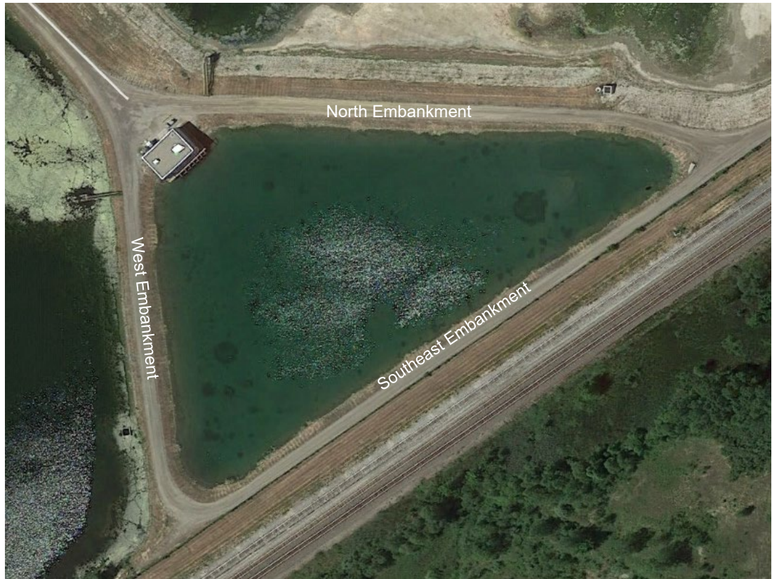
Figure 6. Clear Water Pond Embankment Terminology
