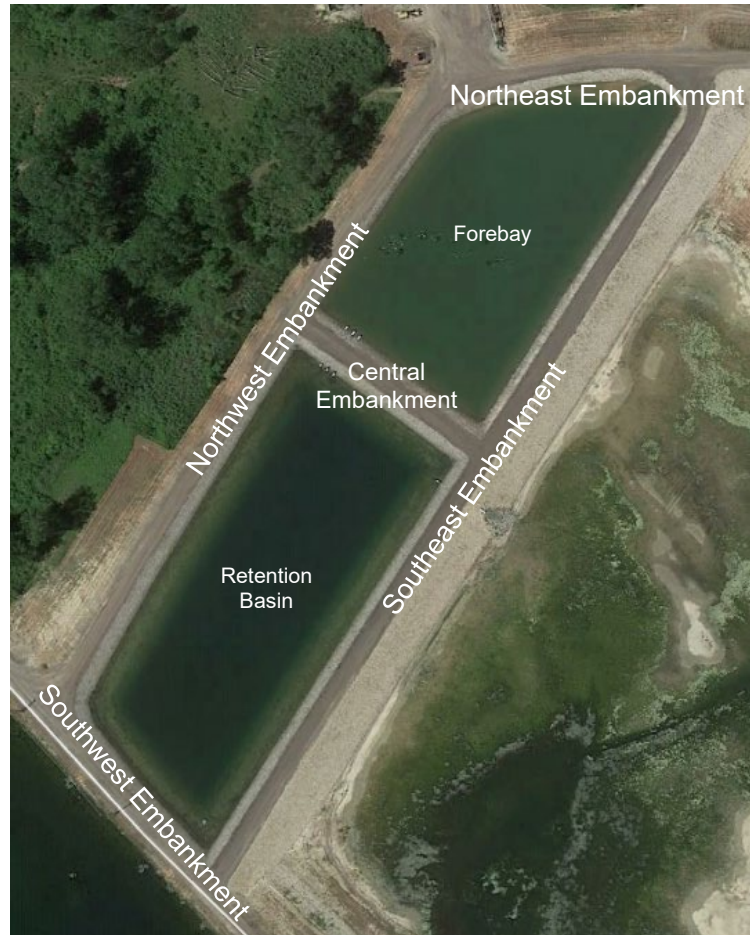
Figure 4. Forebay and Retention Basin Embankment Terminology
