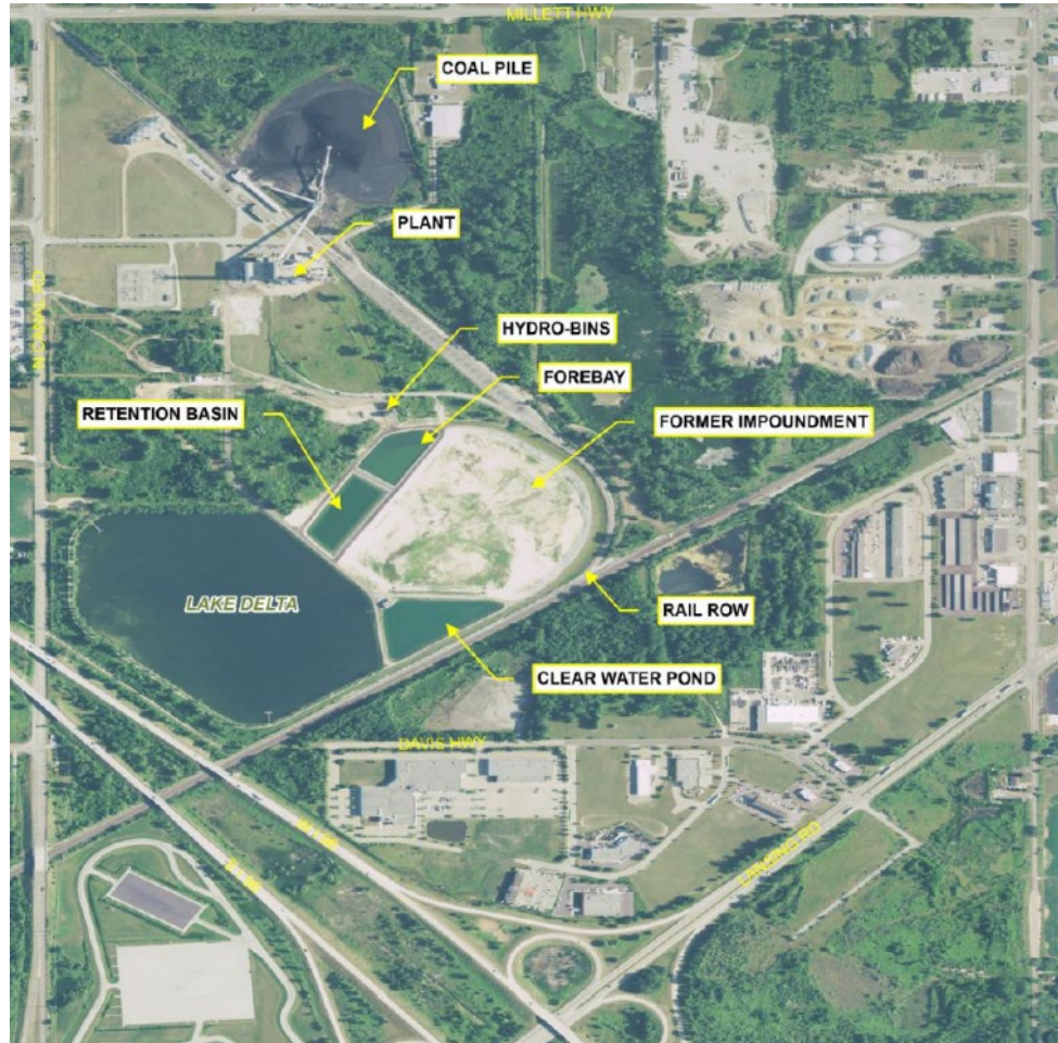
Figure 2. Erickson Power Station Site Configuration
