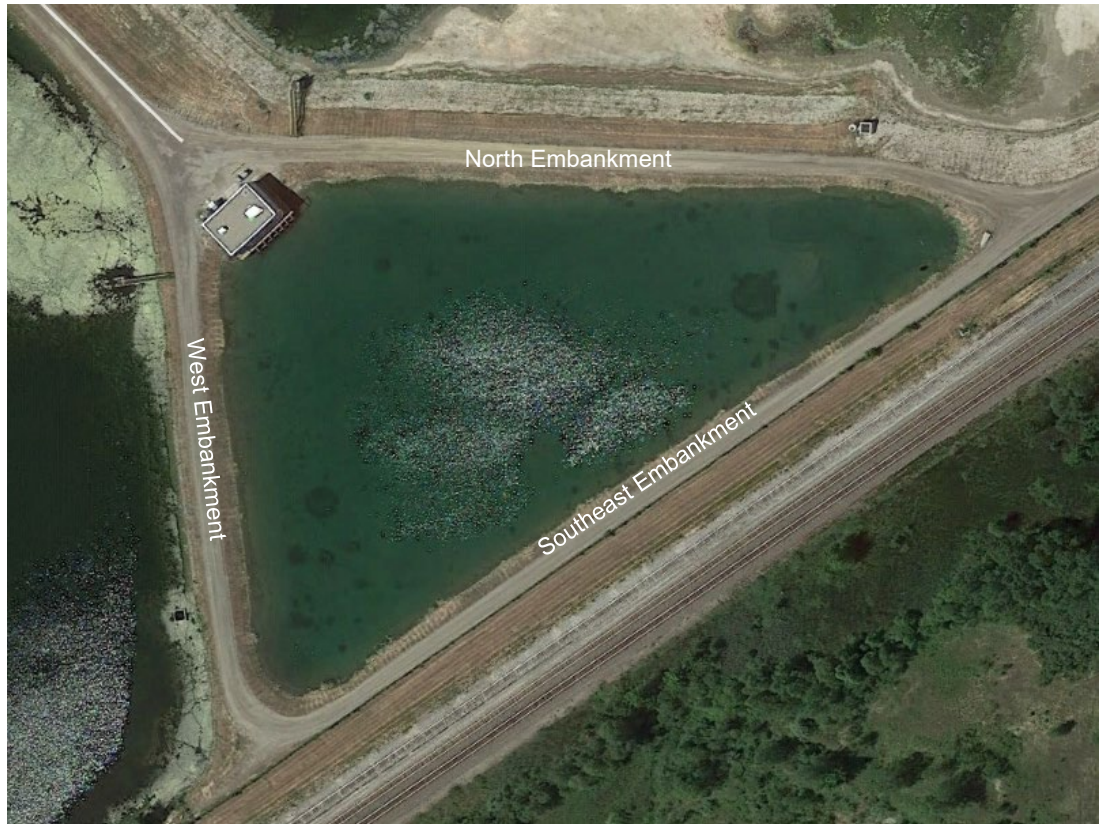
Figure 6. Clear Water Pond Embankment Terminology
