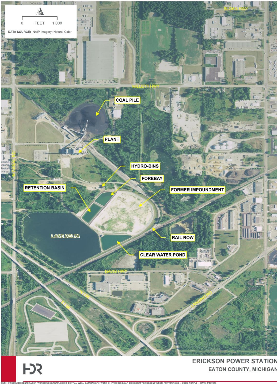
Figure 2. Erickson Station Facility Layout
